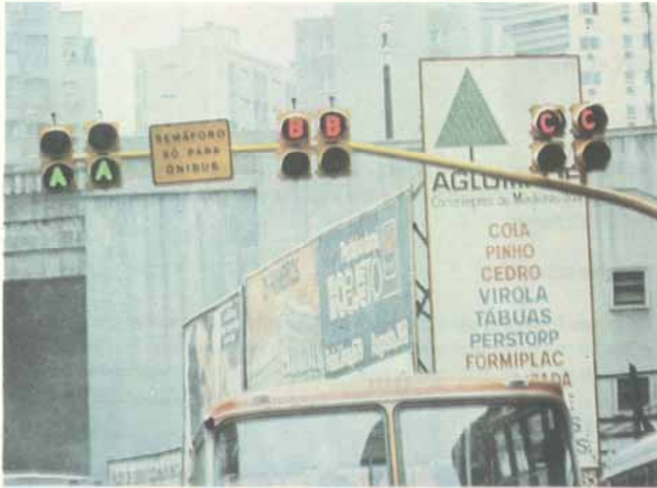
SIGNAL HEADS USED TO CONTROL BUS DEPARTURES
